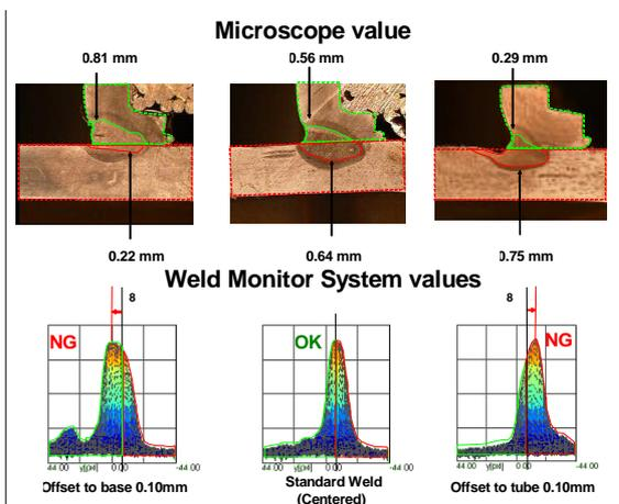
Fig. 6: Visualization of weld offset in 3D Display of monitoring system.
