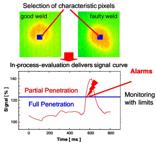
Fig 4: Principle of Monitoring with PD2000
