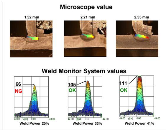
Fig. 5: Visualization of penetration in 3D display of monitoring system as function of laser power.
