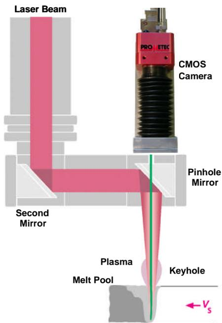
Fig. 3: Setup of a Camera based Inline Weld Process Monitoring on a CO<sub>2</sub> laser
