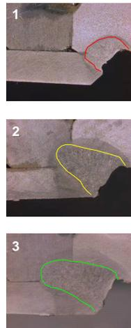
With the selected evaluation methods, a strong linear relationship between penetration and signal height was found. This is confirmed through calculation of the Pearson coefficient (Pearson product-moment correlation coefficient) which equaled 0.8. This coefficient indicates the strength and direction of a linear relationship between two random variables. The closer it is to either -1 or 1, the stronger the correlation between the variables.
