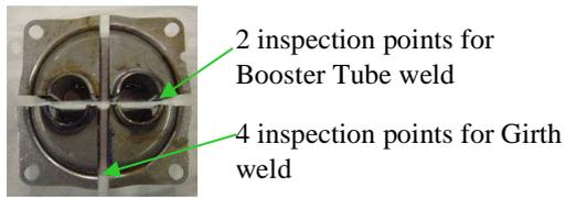
Fig. 2: cross sections of welds
