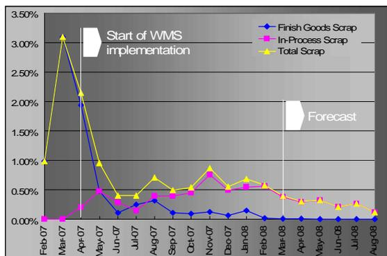
Fig. 8: Scrap rate before and after implementation of Weld Monitoring System
