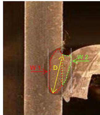
Fig. 1: weld nugget with geometrical requirements
