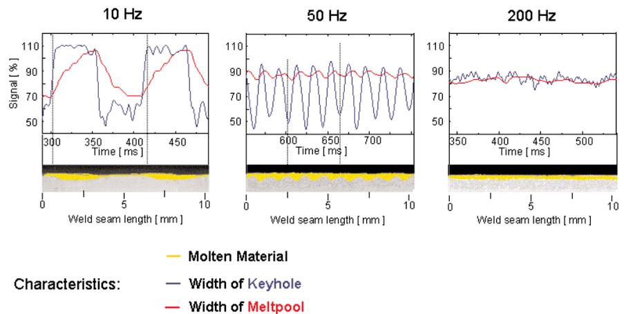
figure 7: Penetration depth and melt pool excitation
