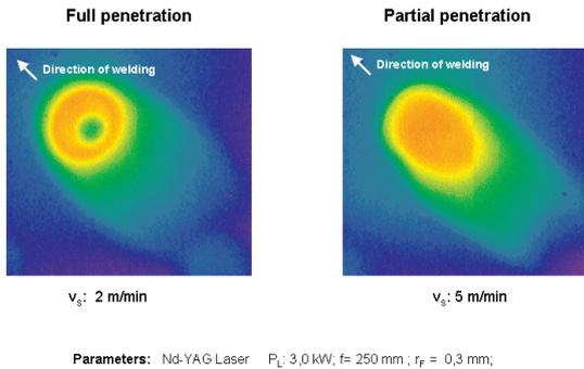
figure 2: Full and partial penetration during laser beam welding with ND-YAG lasers
