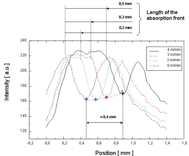
figure 4: Comparison of cross-sections through the intensity distribution in the direction of welding speed
