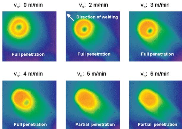
Parameters: Nd-YAG-Laser P<sub>L</sub>: 3,0 kW; f = 250 mm; r<sub>f</sub> = 0,3 mm;
