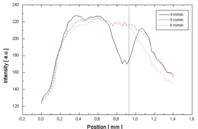
figure 5: Cross-sections through the intensity distribution in the direction of welding speed for full and partial penetration
