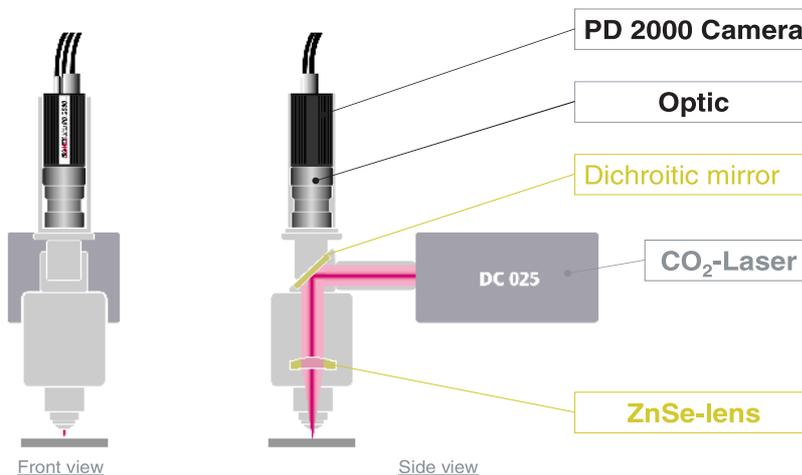
Figure 4: Monitoring setup for cutting with a CO<sub>2</sub>-laser beam and a ZnSe-optic
