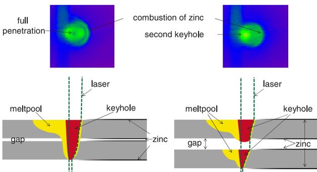
Parameter: Nd-YAG-Laser;  $P_L$ : 4 kW; f: 200 mm;  $v_s$ : 3m/min;  $r_f$ : 0,6 mm; overlapped joint
