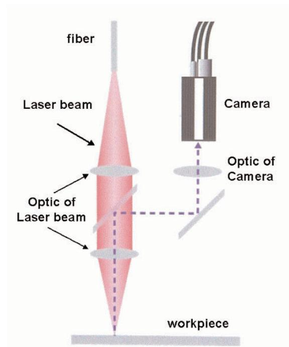
Figure 1: Monitoring setup for a Nd-YAG Laser
